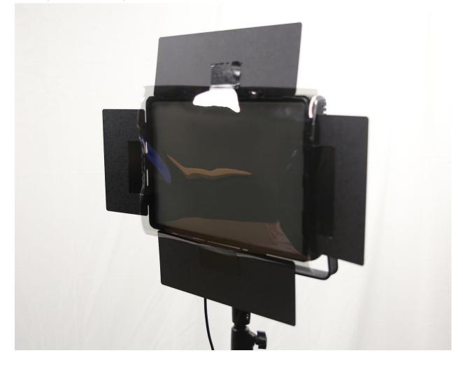
The room itself must be dark, to produce a uniform black background. This means that you must use a strong light to illuminate the object clearly. Using a strong light is also important because, when shooting, the camera must use a small aperture to put the object in a clear depth of field. The example light is covered by a polarized filter and uses LEDs so the heat from the light does not degrade the polarized film. Be aware that heat from strong lights can damage polarized film.
