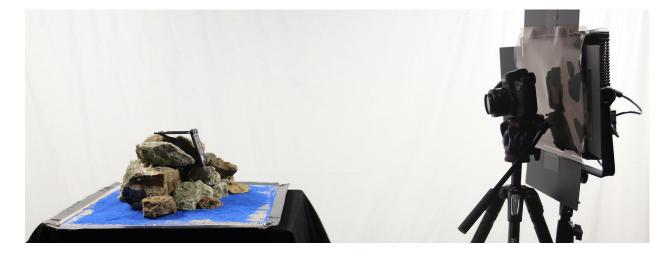
To cover all parts of the object, you must move the camera vertically. Be sure to move the light and camera together.
