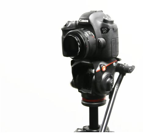
Fix your camera to a tripod and only move it vertically via the tripod. The example uses a Canon 6D. A lens with a fixed focal length will produce better results than an equivalently priced zoom lens. However, the zoom lens is more flexible because it can frame specific smaller details. A close shot session requires a lot of photos, so it is time consuming. If you plan to use tileable materials on the object, a close shot session is likely to be unnecessary.
